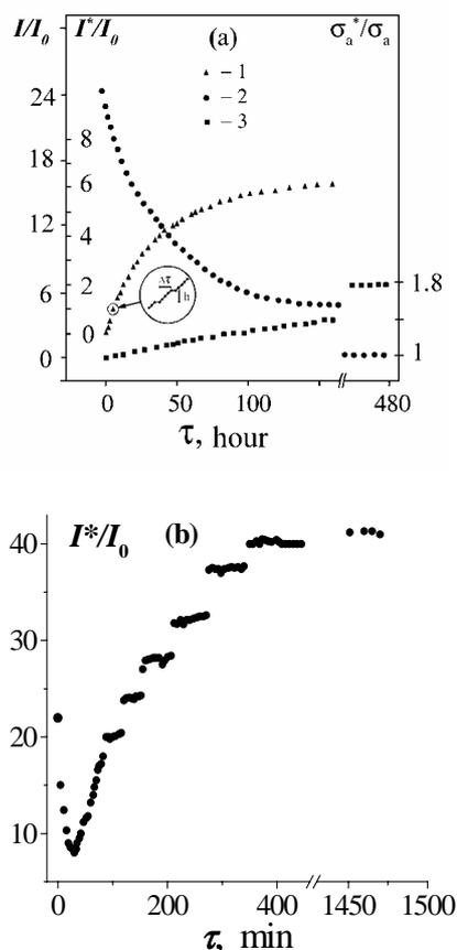
Fig. 3. The intensity of CESR signal from non- ( $I/I_0$ ) and intercalated ( $I^*/I_0$ ) parts of HOPG plate and  $\sigma_a^*$  (3) (the sample A) vs. exposure time,  $\tau$ , in  $\text{SbF}_5$  atmosphere. (a):  $c \perp H_{\text{rf}}$ ; (b):  $c \parallel H_{\text{rf}}$ .  $I_0$  ( $\sigma_a$ ) is the intensity of a standard ESR signal (graphite basal plane conductivity).
