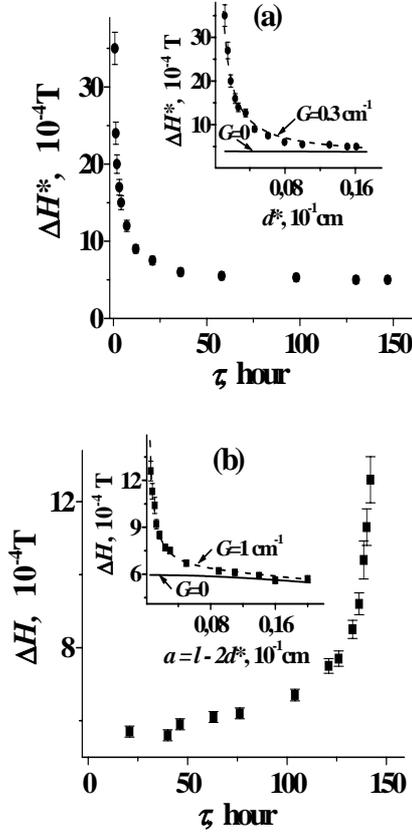
Fig. 2. The linewidth of CESR signal from non- (a) and intercalated (b) parts of HOPG plate (the sample B) vs. exposure time,  $\tau$  in  $\text{SbF}_5$  atmosphere. The experimental (dots) and theoretical (lines) values of linewidth vs. thickness of the non-intercalated ( $a=1-2d^*$ ) and the intercalated ( $d^*$ ) graphite are presented in the corresponding inserts.
