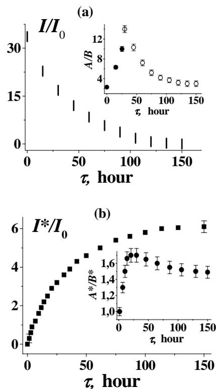
Fig. 1. The CESR lineshape parameters of non-intercalated (a) and intercalated (b) parts of HOPG plate (sample B) vs. exposure time,  $\tau$ , in  $\text{SbF}_5$  atmosphere.  $I_0$  is the intensity of the standard ESR signal.
