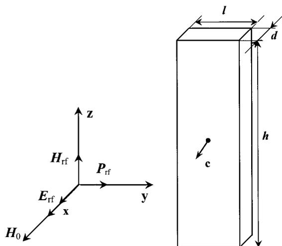
Fig. 1. The orientation of the HOPG plate with respect to the external magnetic field  $\mathbf{H}_0$  and the cavity axis.  $\mathbf{H}_{\text{rf}}$ ,  $\mathbf{E}_{\text{rf}}$  and  $\mathbf{P}_{\text{rf}}$  are the magnetic and electric components of the radio-frequency field, and the Poynting vector in an unloaded rectangular cavity, respectively
