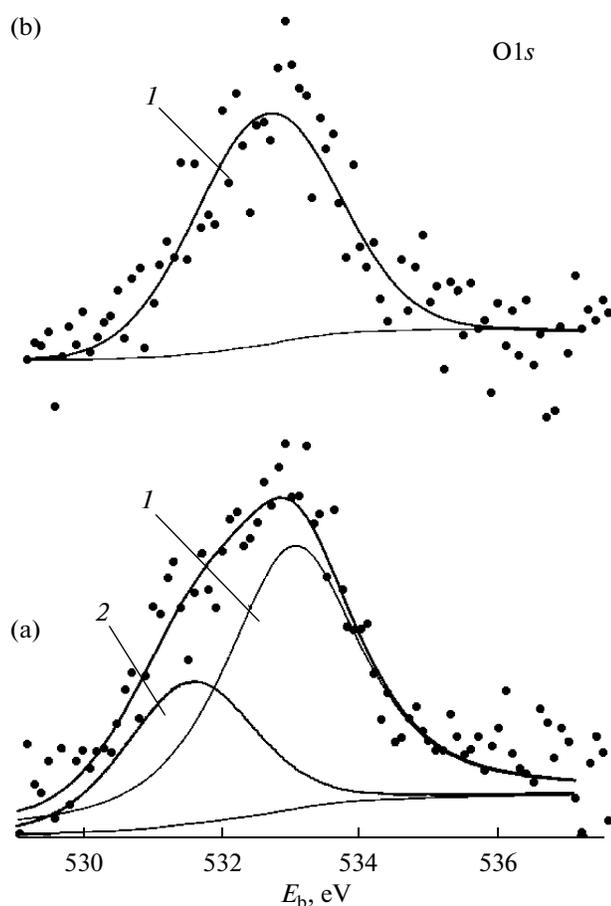
**Fig. 2.** The O1s XPS spectra of (a) the initial ACF and (b) the ACF annealed at 850°C: (1) the oxygen line of  $-OR$  groups ( $R$  is a hydrocarbon radical or H) and (2) the oxygen line of the carbonyl group.
