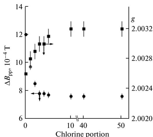
**Fig. 9.** The  $g$ -factor values and the CESR signal widths ( $\Delta B_{pp}$ ) as functions of the number of chlorine portions admitted into the reactor with ACF.
