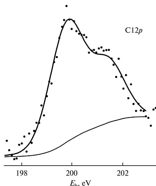
**Fig. 8.** The Cl2p XPS spectrum of chlorinated ACF.
