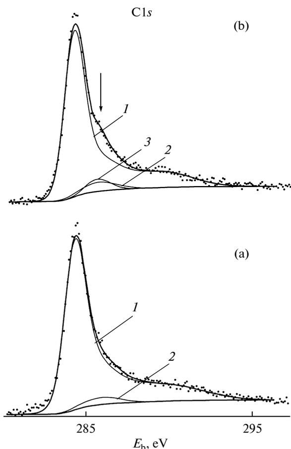
**Fig. 7.** The C1s XPS spectrum of ACF (a) before and (b) after chlorination: (1) spectrum component caused by the carbons of nanographites, the aliphatic fragments of the fiber, surface hydrocarbon impurities, and lines due to the  $\pi \rightarrow \pi^*$  excitation; (2) spectrum component corresponding to the carbon of C–OR groups, where R is a hydrocarbon radical or H; and (3) spectrum component corresponding to the carbon bound to chlorine.
