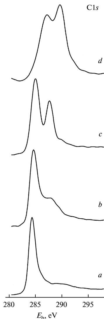
**Fig. 4.** Smoothed C1s XPS spectra of (a) the initial ACF and the ACFs fluorinated at (b) 100, (c) 155, and (d) 300°C.
