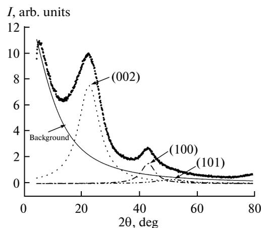
**Fig. 3.** X-ray diffraction spectrum of ACF and its deconvolution into three Lorentzians corresponding to the (002), (100), and (101) reflections.
