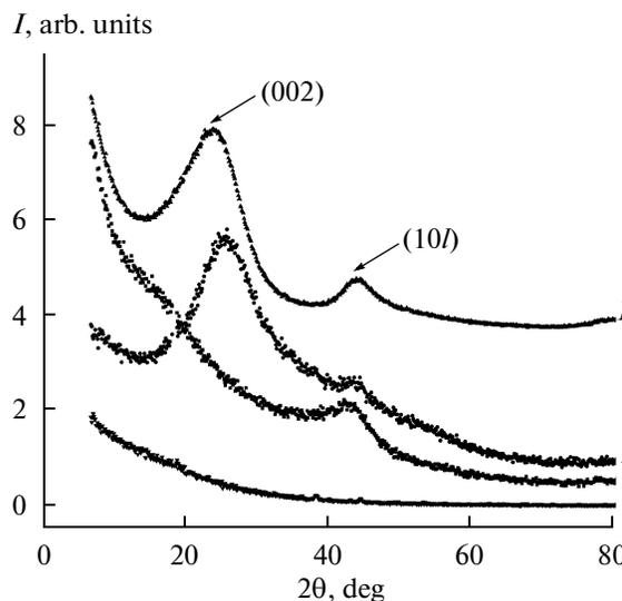
**Fig. 5.** X-ray diffraction spectra of (1) the initial ACF and the ACFs fluorinated at (2) 100, (3) 155, and (4)  $>300^{\circ}\text{C}$ .
